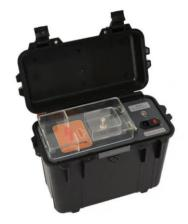
It is working together with GD-4133 Cable Fault Detector, used for detecting high
